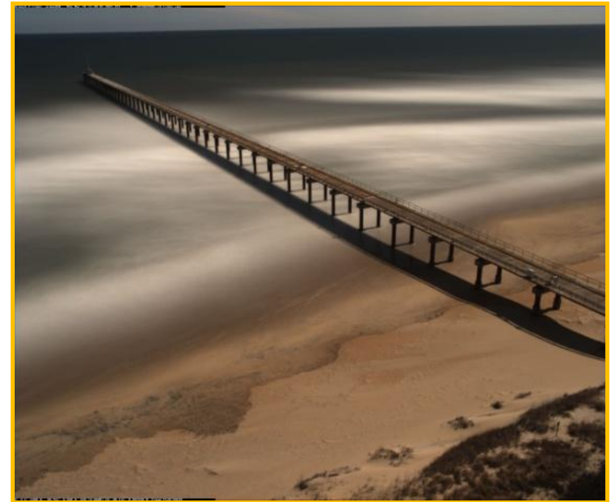
Time-averaged image created from video footage from the Video Tower at FRF. Once each image is georectified using ground control points, nearshore characteristics can be quantified.
