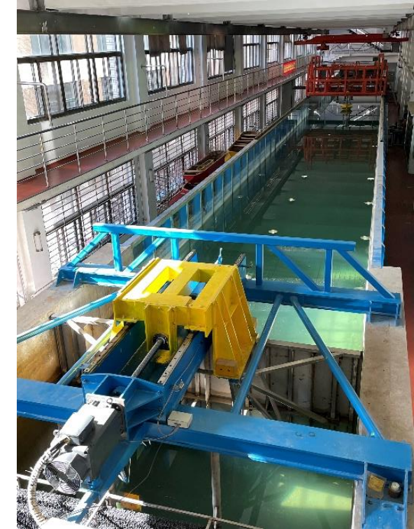
Wave tank with (69m, 4m, 2.5m) Dalian University of Technology
