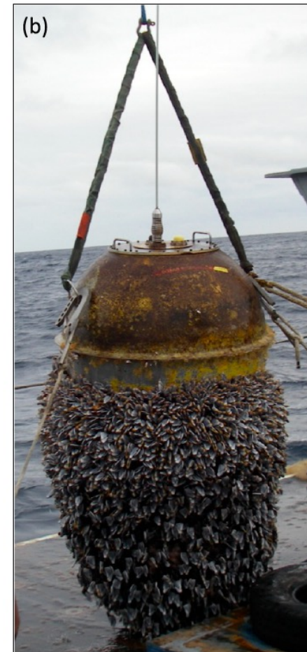
FIG. 2. Before and after pictures of the 0.9-m-diameter waverider buoy at Ocean Station P . (a) Newly painted buoy on deck before deployment in October 2012, and (b) biofouled buoy after recovery in January 2015.
