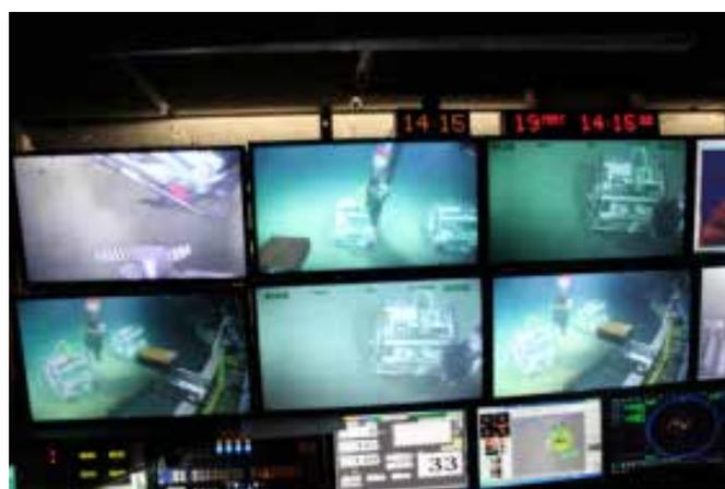
Above: Recovery of benthic chamber 2 and deployment of benthic chamber 1 on May 19 as viewed on the giant multiple screens in the control room of the ROV ISIS on board RRS *James Cook*.
