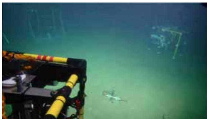
Figure 2. The experimental site just prior to CO<sub>2</sub> release. Clockwise from lower left are the sediment profiler (on the ROV), a hydrophone wall, a BBL lander, and a sediment pH optode.
