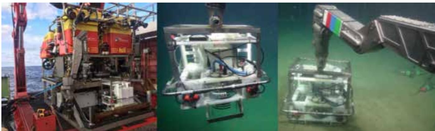
Above, left: Benthic chamber on the front porch of the ROV ISIS, ready for deployment. Middle: benthic chamber about to be placed by ROV ISIS in the seafloor in the vicinity of a CO<sub>2</sub> bubble stream. Right: Recovery of a benthic chamber by the mechanic arm of the ROV ISIS after a 2-day deployment.
