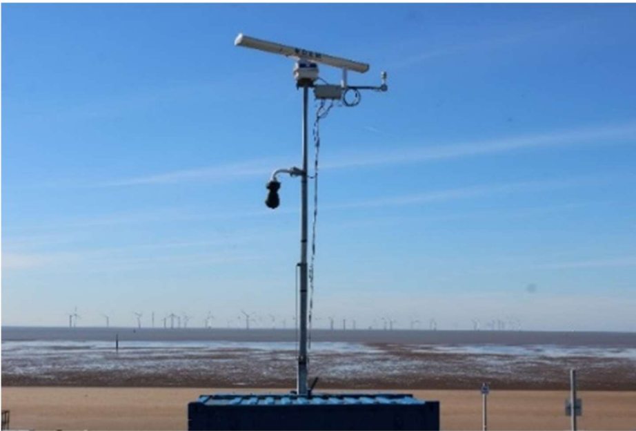
Figure 13: Radar survey platform (Marlan Maritime Technologies Ltd)
