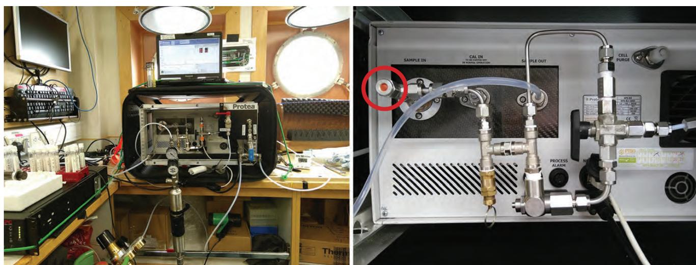
Figure 18: Gas analyser used for on board analysis of the gas composition. Red circle on the right-hand image indicates the sampling port used for retrieving discrete gas samples for Kr,  $\delta^{13}\text{C}$  and  $\delta^{18}\text{O}$  analysis. Images courtesy A. Flohr.
