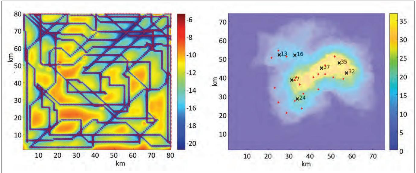
Figure 27: Left - Optimal path taken by an AUV<sup>17</sup>. Right - Optimal sensor placements using simulation of 36 leaks at different locations. Sensors placed such that any of 36 leaks would be detected while keeping the number of sensors minimal<sup>16</sup>.
