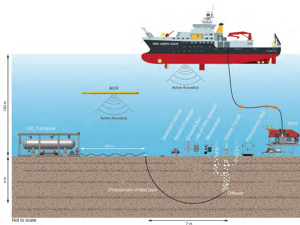
Figure 2: Schematic showing the STEMM-CCS controlled release experiment. Image courtesy C.Pearce, NOC.
