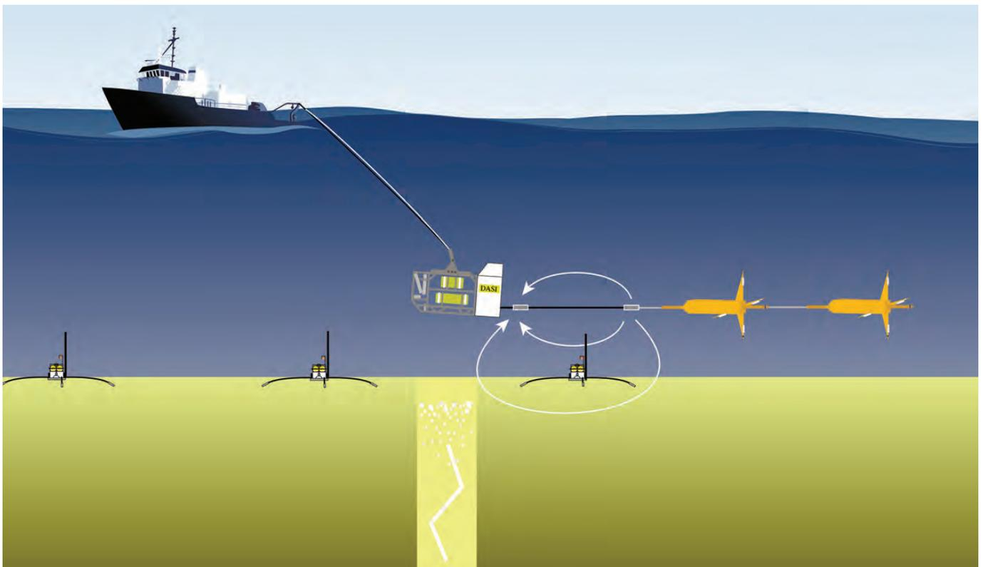
Figure 15: Deep-towed electromagnetic experiment sketch (not to scale) including a source that injects an electric current (white lines), towed receivers (orange tow bodies) and ocean-bottom receivers across a vertical fluid conduit (indicated by white arrow and bubbles). Image adapted from K. Weitmeyer and finalised by K. Davis.
