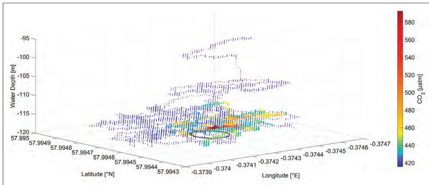
Figure 20: Map of the distribution of dissolved carbon dioxide measured in the water column above the sub-seabed CO<sub>2</sub> injection point (black ellipse) at the Goldeneye experimental site. Rate of CO<sub>2</sub> injection = 50 L/min. Image courtesy J. Gros (GEOMAR).
