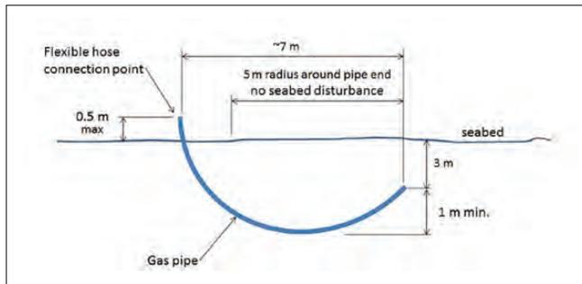
Figure 5: Illustration of gas release pipe geometry used in the experiment.
