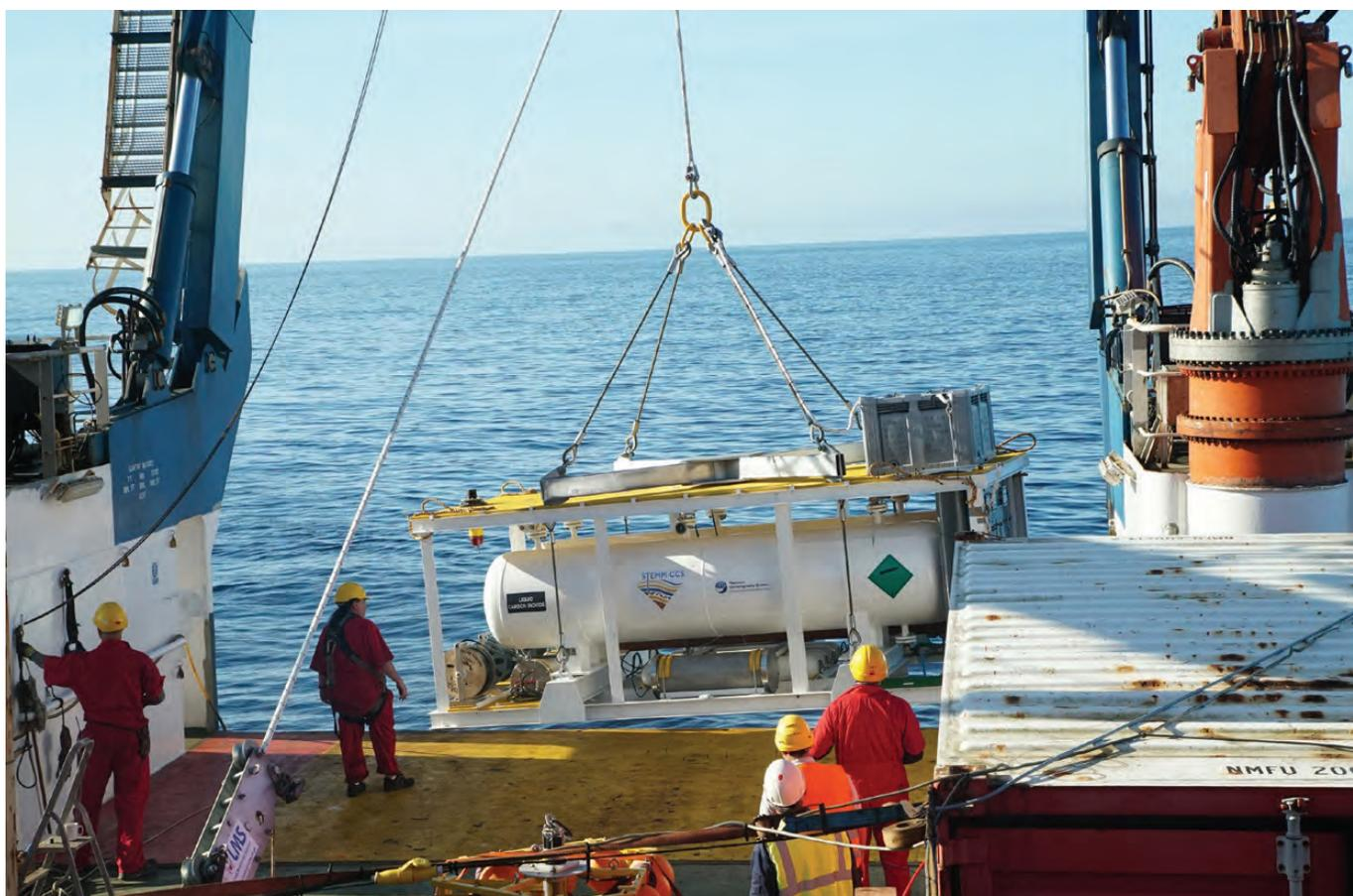
Figure 7: Deployment of the bespoke gas storage and release system from the back deck of RRS James Cook.
