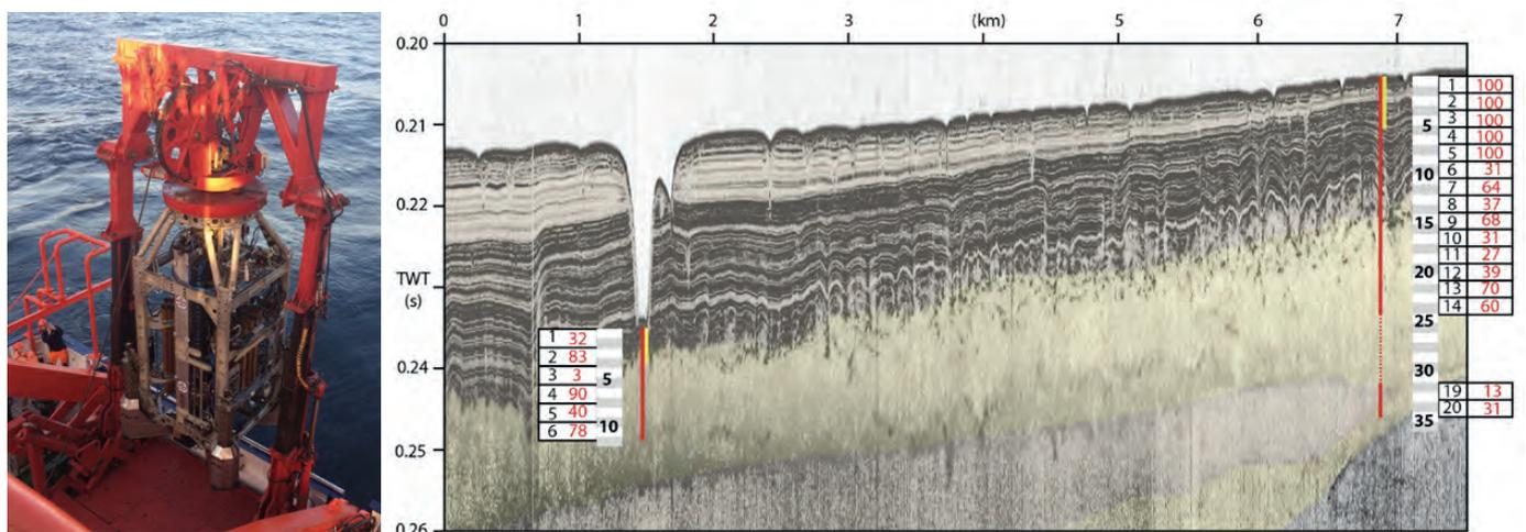
Figure 16: Left: RockDrill2 deployment during *Maria S. Merian* cruise MSM78 <sup>7</sup>. Image courtesy J.Karstens. Right: Sediment echosounder profile showing the relative location of the drill site in the Scanner pockmark and the reference site. Red lines show core recovery. The deep depression of the seafloor is the Scanner pockmark <sup>7</sup>.
