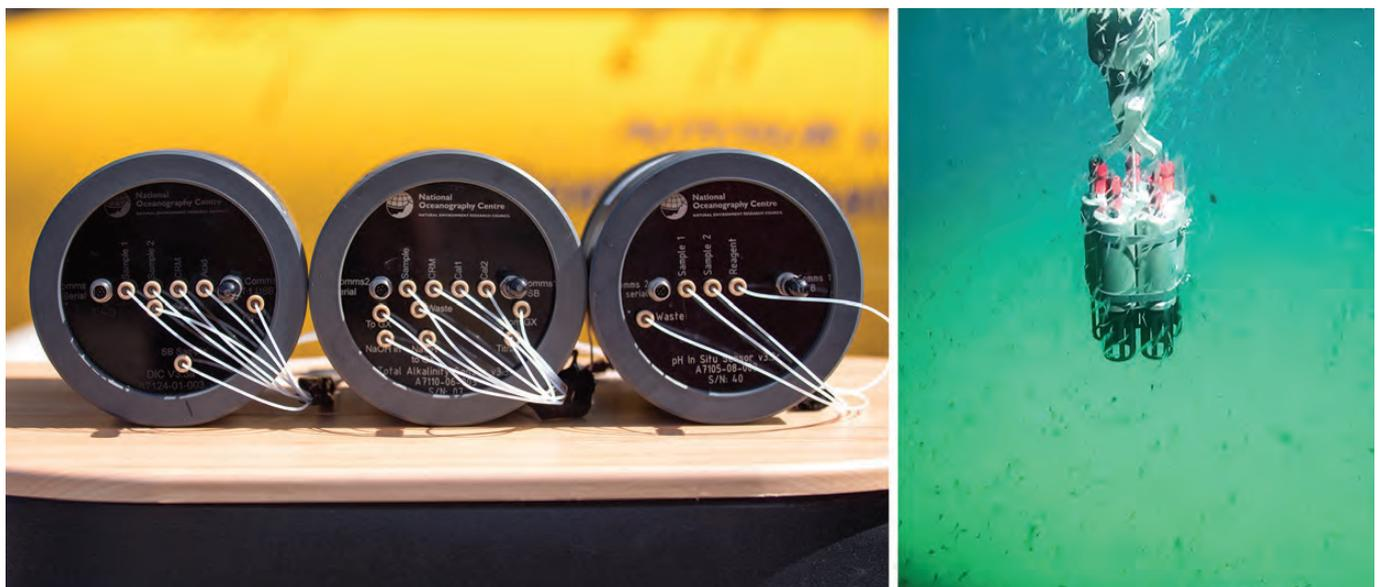
Figure 21: Novel Lab-on-Chip (LOC) sensors (left) and dissolved oxygen (DO) optodes for autonomous in situ measurement of pH, TA and DIC integrated into landers and ROVs. Images courtesy NOC.
