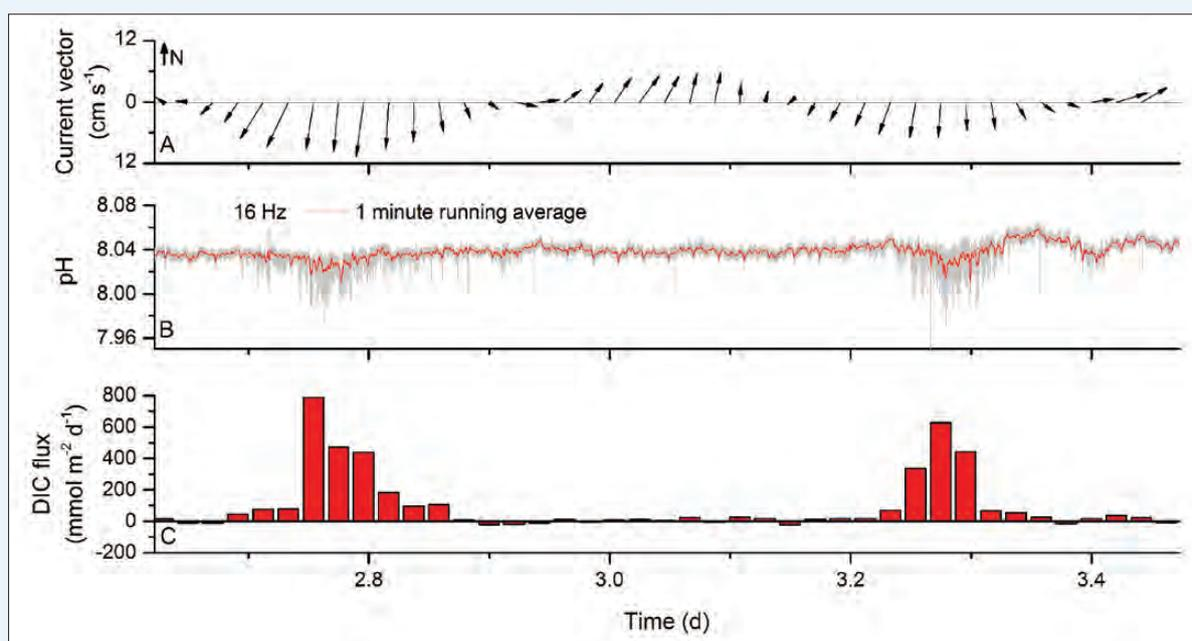
Above: Detection and quantification of the CO<sub>2</sub> bubble stream at the lowest release rate (5.7 kg d<sup>-1</sup>) by pH eddy covariance. A) Current vector of water velocity and direction relative to north; B) pH time series with anomalies due to the CO<sub>2</sub> bubble stream; C) DIC flux calculated with pH eddy covariance.
