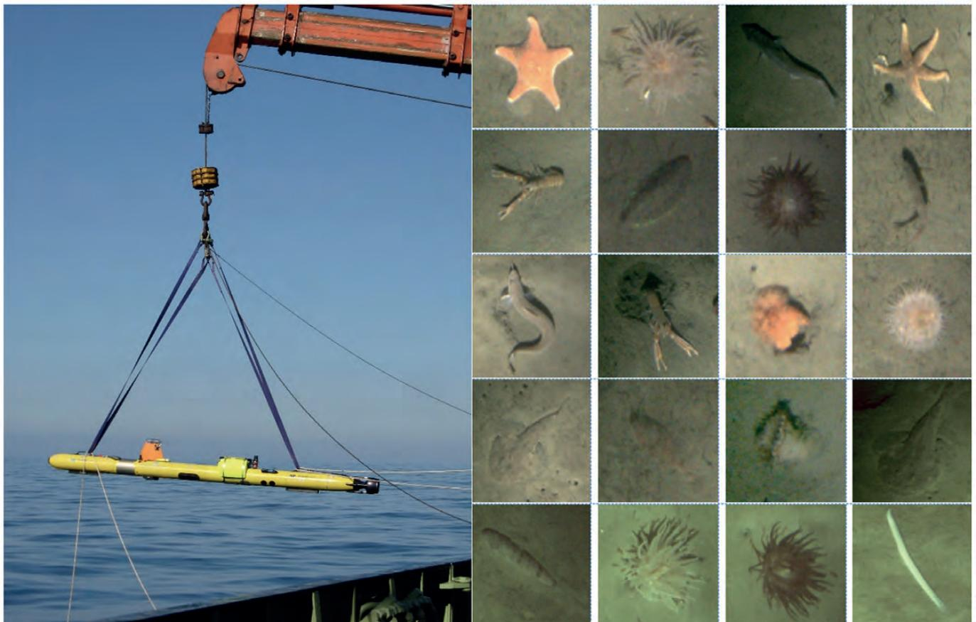
Figure 11: The Gavia Autonomous Underwater Vehicle deployed at the Goldeneye site (left), and a series of representative benthic megafauna specimens, photographed by the Gavia AUV (right)
