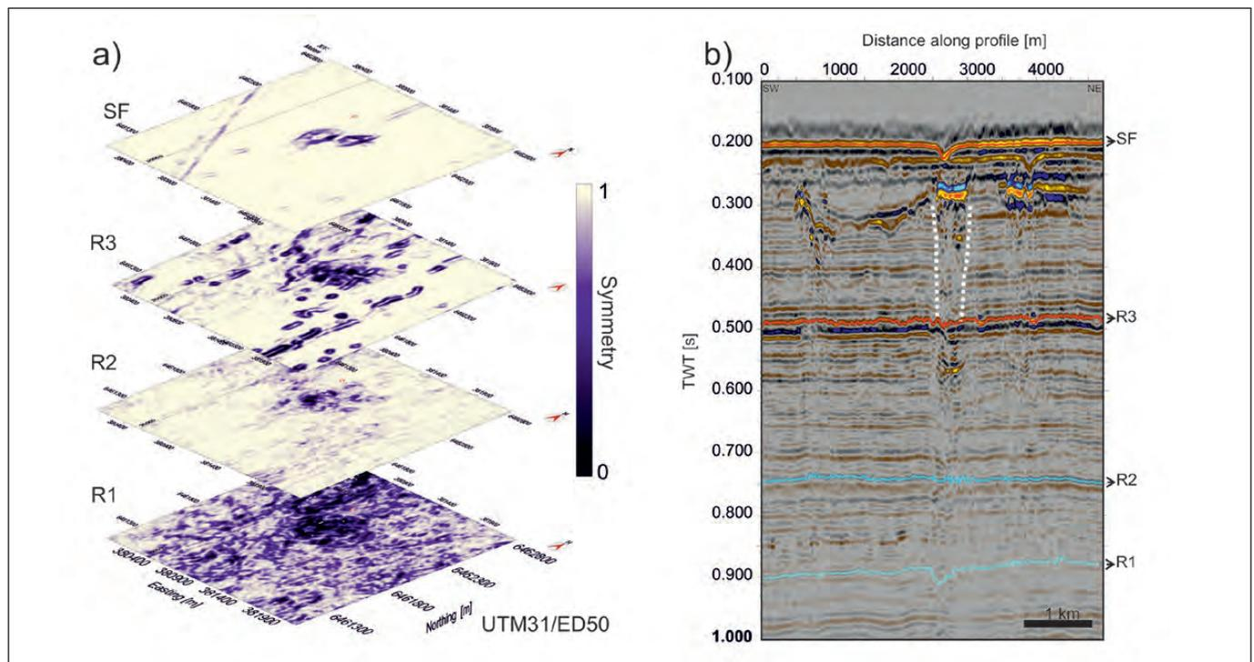
Figure 14: 3D seismic image of the pipe structure underneath the Scanner pockmark reaching down to about 0.7 s two way travel time (TWT) or approximately 600 m (right) and slices through a coherence cube (left) at the same location showing the three-dimensional geometry of the pipe depth at different depth (for depth see labels on the right figure). From Böttner et al., 2019<sup>5</sup>.
