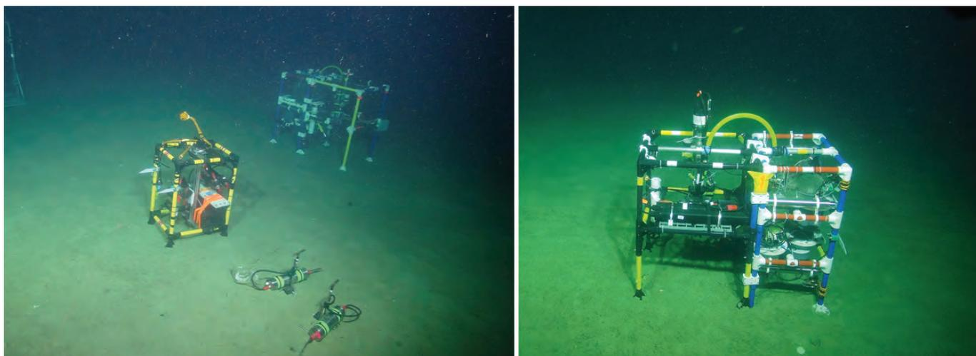
Figure 22: Sediment microprofiler (left) and benthic boundary layer lander (right) with integrated novel electrochemical, optical, and LOC wet chemical sensors for the determination of fluxes across the sediment-water interface. Images courtesy NOC/JC180.
