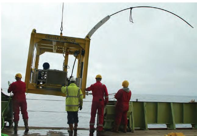
Figure 6: Deployment of the drill rig from RRS James Cook.
