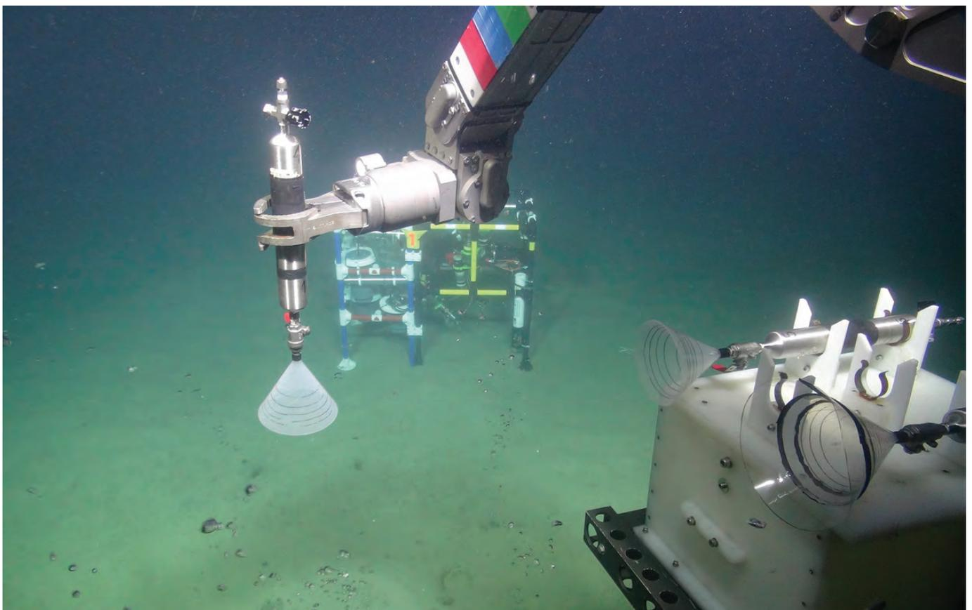
Figure 17: Collection of gas samples using a gas bubble sampler deployed from the remotely operated vehicle. The time taken to fill the funnel with gas was noted to derive an approximate estimate of the leakage rate. Image courtesy NOC/JC180.
