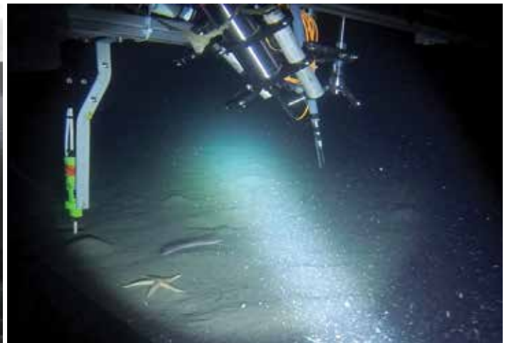
Above, left: the MPI benthic lander on the back deck, ready for deployment. Above right: Fast-response sensors measure turbulence at the seafloor.
