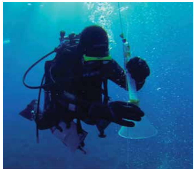
Figure 1. A scientist collecting gas bubbles that were later analysed for their chemical composition. Evolution of the average gas bubble composition as it rises through the water column represents a fingerprint of the underlying mass transfer processes, and in particular of the rapid dissolution of CO 2 .
