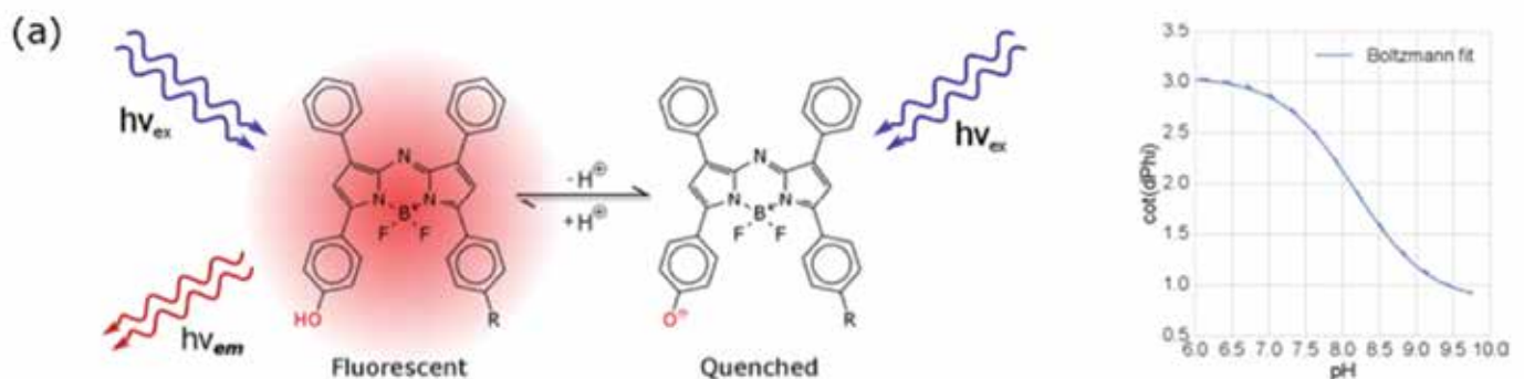
Figure 1: (a) Chemical structure of the employed fluorescent indicators showing the acid-base equilibrium; (b) Example of the calibration curve showing experimental data (points) and the Boltzmann sigmoid fit.
