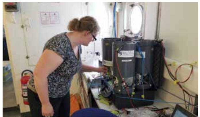
Above: NOC's Allison Schaap monitors lab-on-chip chemical sensors aboard RV Poseidon as they continuously measure seawater composition.
