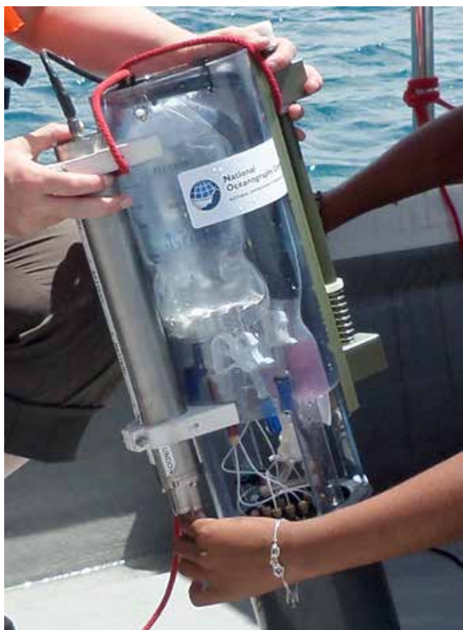
Figure 2: Complete lab on chip system with reagents in a transparent housing above the sensor, about to be deployed off the side of a small ship.
