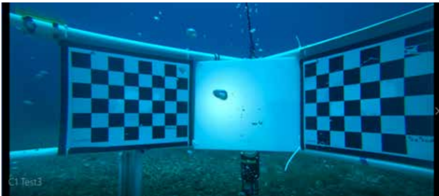
Bubbles rising against the backdrop of the scale board, as seen by a camera on AOL. Squares on the scale board are 5cm x 5cm.
