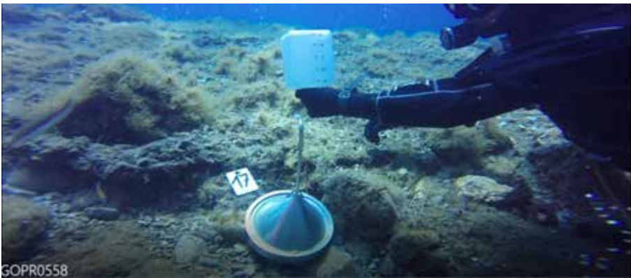
Andrea Fogliozi carrying out a "bubble box" experiment. It took this single vent just 53 seconds to fill the 2 litre box.
