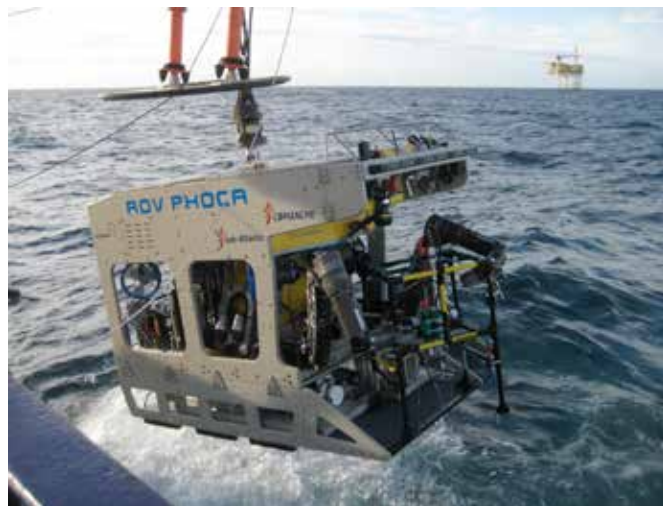
Figure 2. Retrieval of the oxygen and pH eddy covariance system from the seafloor by a remotely operated vehicle. The Goldeneye platform is visible on the horizon.
