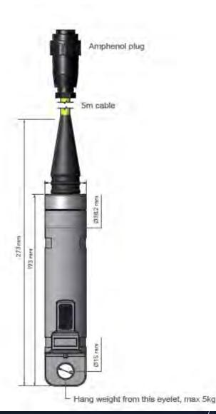
Oxygen:  $O_2$  Concentration Air Saturation Operation Range:  $0-800 \mu M^{11}$  0-200% Calibration Range:  $0-500 \mu M^{11}$  0-120% Resolution:  $<1 \mu M$  0.4% Accuracy:  $<8 \mu M$  or  $5\%^{21}$   $<5\%^{31}$
