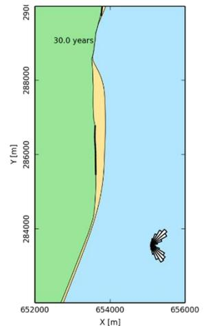
The **conservation equation** for beach sediment expressed in terms of local coordinates states that the change in position of the shoreline ( $d\eta$ ), perpendicular to the local shoreline orientation ( $s$ ) through time ( $t$ ) is a function of the divergence of alongshore sediment flux ( $Q$ ).
